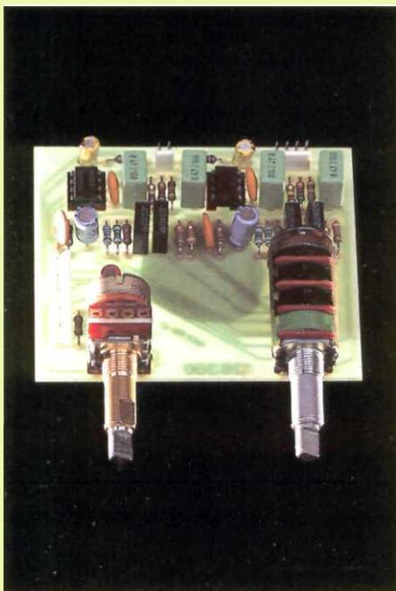
*The compandor circuit and control, the loudness circuit and control, and the balance control are incorporated on this one compact epoxy fibreglas board. As with all circuit boards. It is interconnected with plug-together cables to prevent soldering malfunction.*
