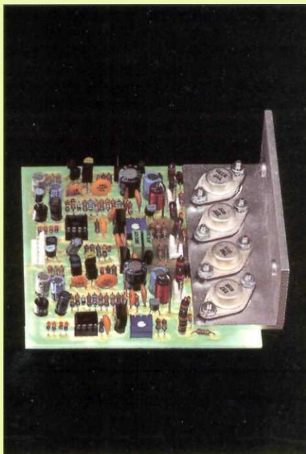
*The power amplifier along with the speaker and music protecting POWER GUARD and SENTRY MONITOR circuits are mounted on this circuit board. Notice the heat sink which is intimately engaged with the entire chassis to rapidly dissipate any heat generated.*
