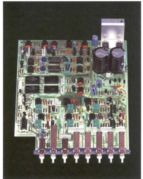
*The main circuit board in the C 33, as with the other boards, is constructed of military grade epoxy fibreglas resin. The photo processed circuit foils are protected from excessive solder, potential short circuits, and destructive circuit bridging by an extra process, screened solder resist. This is another McIntosh practice to protect your musical pleasure and the unit's performance.*
