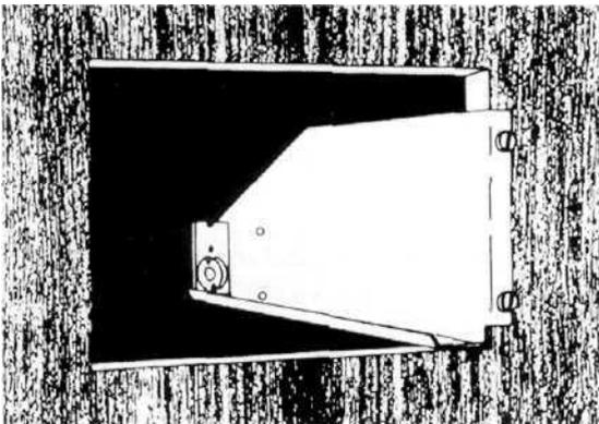
Position the PANLOC shelves inside the cutout with the short flange against the front face of the cabinet panel. Fasten the shelves by inserting two fillister head 6/32 screws through the holes in each of the PANLOC shelf flanges, through the front panel and into the threaded receptacle on the mounting strips.
