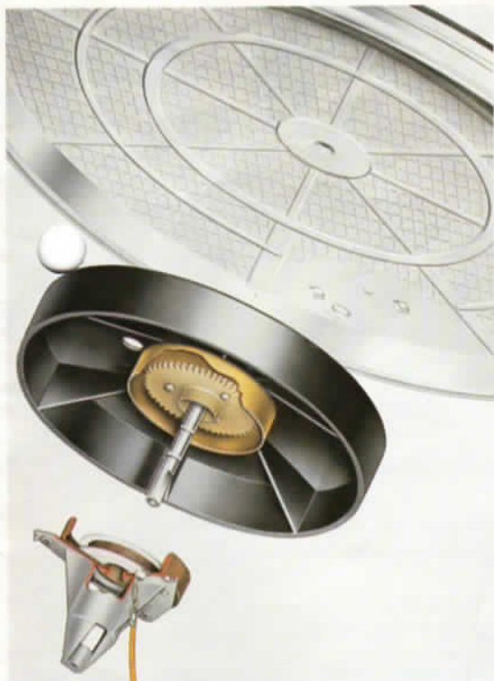
Exploded view of turntable assembly showing speed-sensing tachometer
