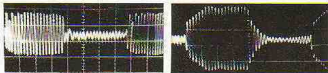
The generally excellent tone-burst response of the Rectilinear system is demonstrated by these bursts at 540 and 10,500 Hz.
