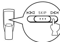
To skip to the beginning of the current track, press the **SKIP**  $\triangleleft \triangleleft$  button once.
