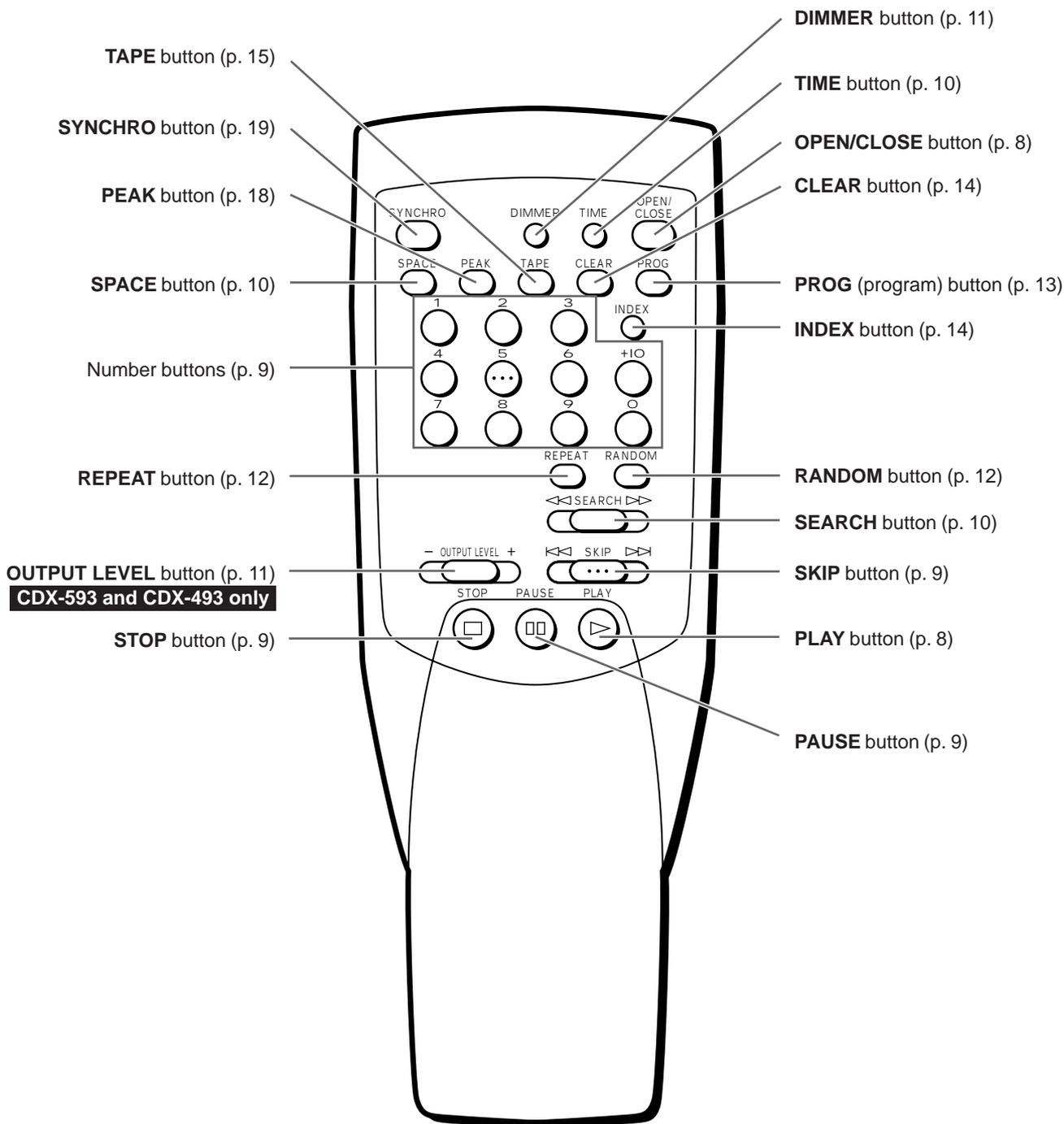
\* The CDX-593 is used for illustration purposes in this manual. Any difference in the operation of other models is clearly indicated in this instruction (for example, "CDX-593 only"). This manual describes how to operate this unit by using the remote control transmitter. To operate this unit from the front panel, use the corresponding buttons on the front panel.
