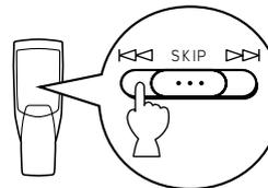
To skip to a preceding track, press the **SKIP**  $\triangleleft \triangleleft$  button repeatedly until the desired track number appears.
