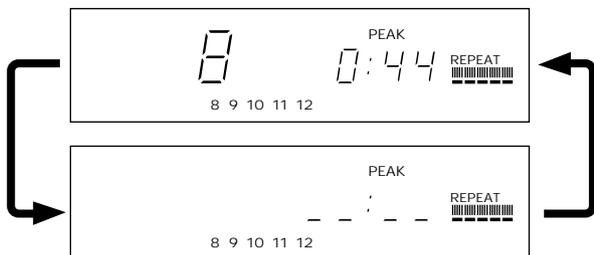
Next, the part where the source level peaks is repeatedly played. Adjust the recording level on the tape deck listening to this sound.
