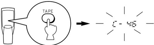
You can select any of four tape lengths by pressing the **TAPE** button.
